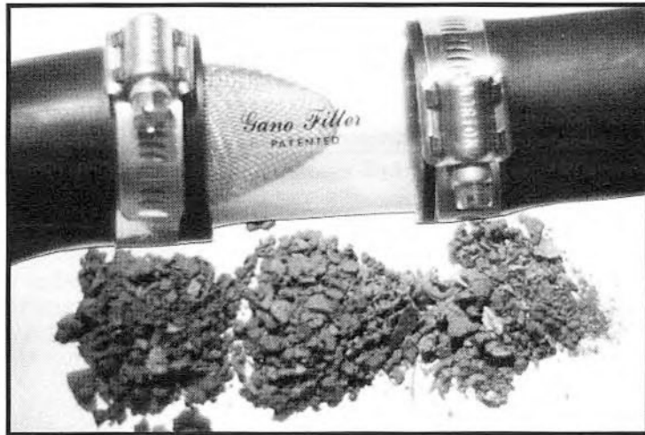
These particles were trapped by the Gano Filter and removed from the cooling system of a 1966 Mustang over a period of one year.
